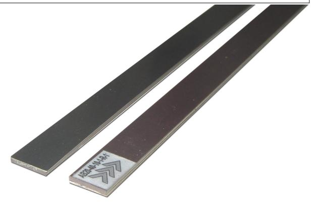
The ELGO magnetic tapes contains digital information, which are necessary for magnetic measurement by ELGO linear encoder types, either as an incremental or absolute code. The tape must be installed along the measuring distance and can be stuck (standard tape construction R) or can also be installed owing to its own magnetization on ferro-magnetic surfaces (when ordered tape construction A).
