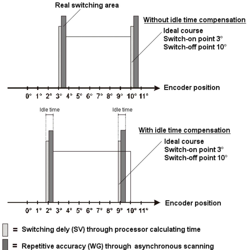
Picture 11: Timing diagram - idle time compensation
