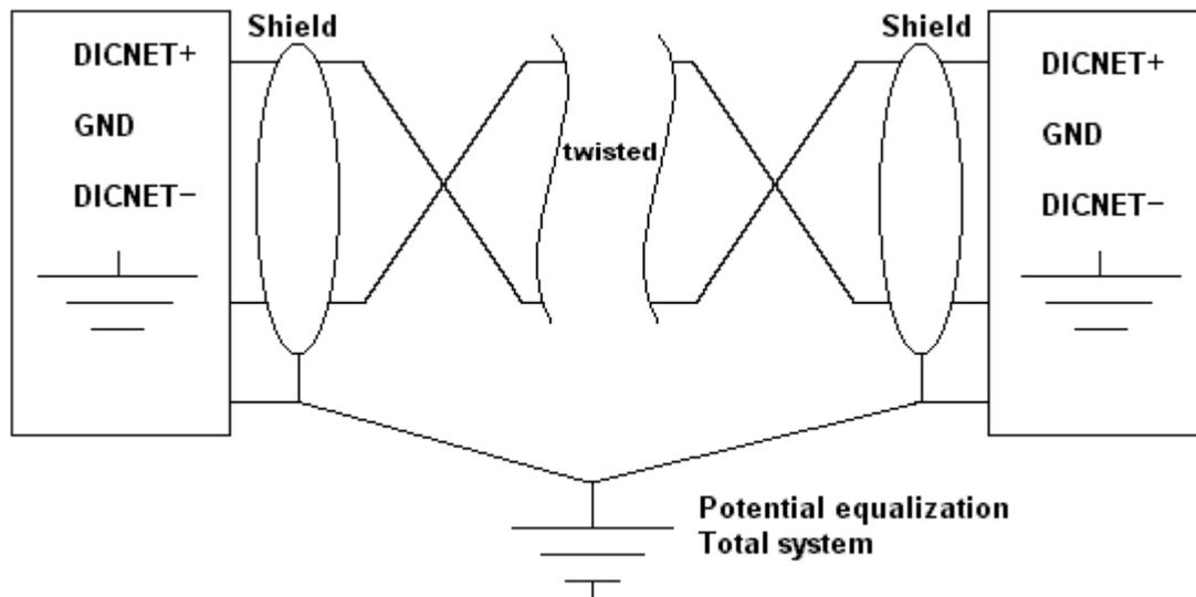
Picture 7: DICNET-wiring
