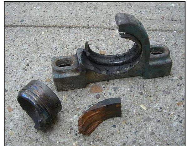
Example of Bearing Failure
