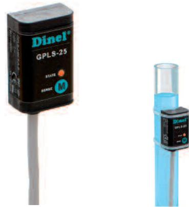
Through wall level switches **GPLS-25** are intended for liquid (conductive and non-conductive) level detection on glass or plastic gauge-pipes, tubes and tanks. The sensitivity and modes (SO – normally open or SC – normally closed) of the switches can be easily set by placing magnetic pen on sensitive spot. The connection is done by means of two wires directly into a circuit with relay or to binary input of control system.
