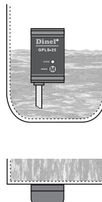
Thru-wall level sensing of liquids in **plastic or glass vessels with flat walls**. The sensor is installed on a clean and degreased surface of the vessel wall. The attachment is done by double-sided adhesive layer. Orientation of the sensor can be arbitrary. Maximum thickness of the vessel wall depends on the detected medium (see technical data); the maximum is 8 mm.
