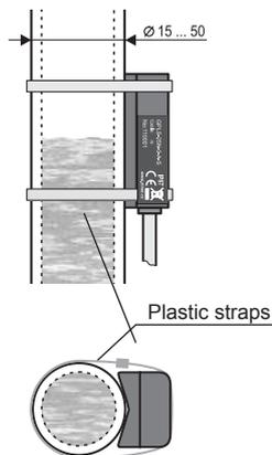
Point level detection on **plastic or glass gauge pipes and tubes**. The sensor is fixed to the gauge pipe or tube by means of two plastic straps (2.5 mm width). The cable should be vertically downwards oriented. The maximum wall thickness of the tube depends on the detected medium (see technical data); the maximum is 8 mm.
